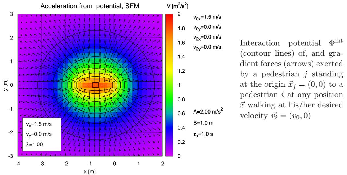
The interaction potential decreases exponentially with the semi-minor axis  $b$  of an ellipse (cf figure) with
