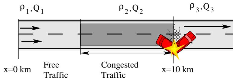
On the remaining left lane,  $Q_{\text{out}} = 1800 \text{ veh/h}$  can pass the bottleneck. The traffic demand for the whole direction (both lanes together) is given by
