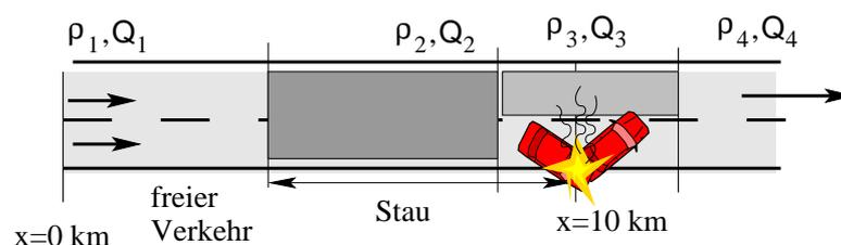
Solve the following questions using the LWR with the triangular fundamental diagram with the parameters  $l_{\text{eff}} = 8 \text{ m}$ ,  $T = 1.5 \text{ s}$ , and  $V_0 = 28 \text{ m/s}$ .
