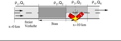
Solve the following questions using the LWR with the triangular fundamental diagram with the parameters  $l_{\text{eff}} = 8 \text{ m}$ , T = 1.5 s, and  $V_0 = 28 \text{ m/s}$ .
